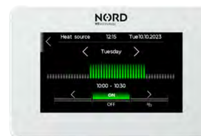
Setting the operation schedule of the EcoHeat heat pump
